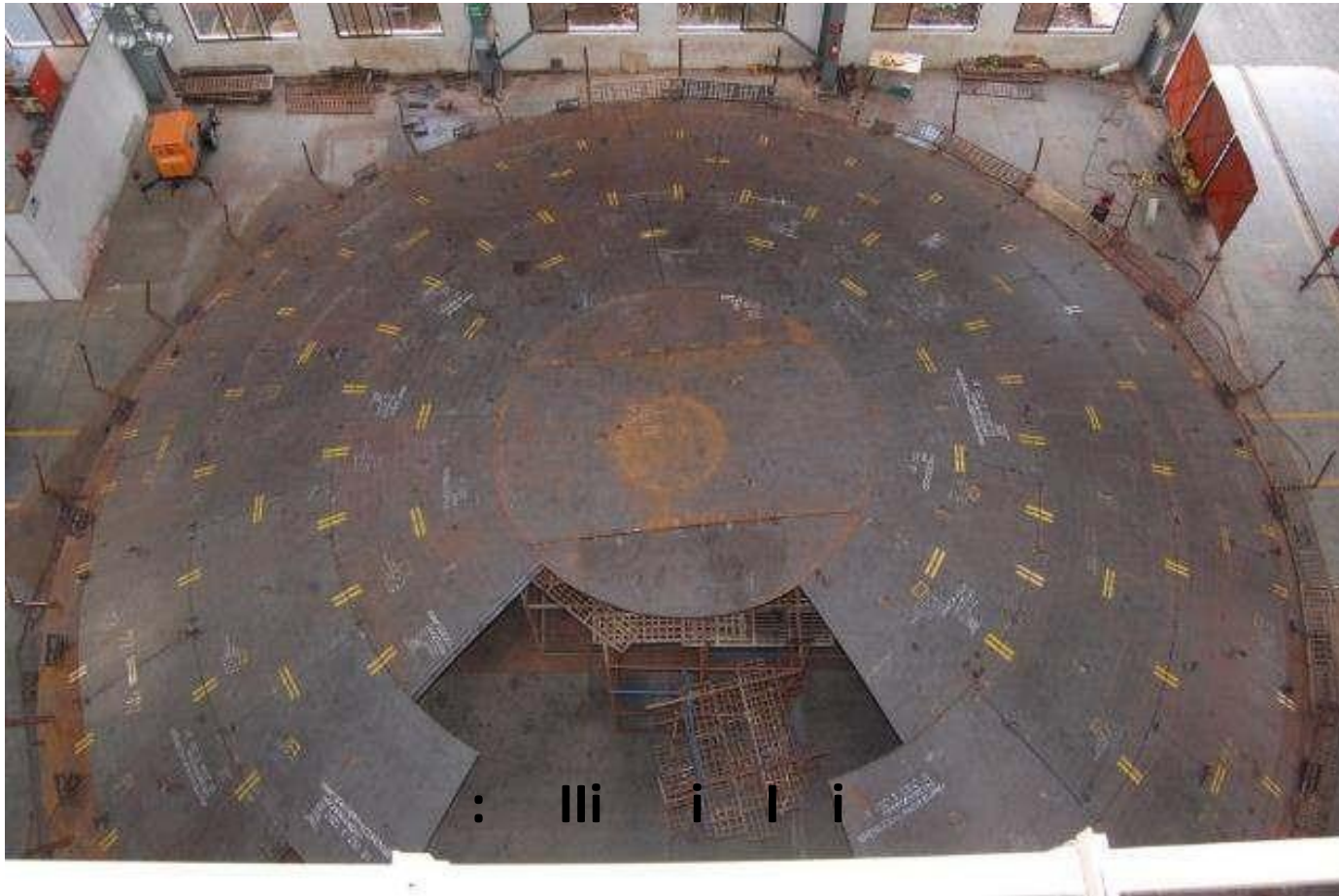
Fabrication & Mock up Assembly of Ellipsoidal Dish End
