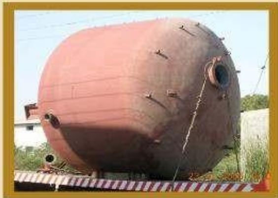
Pressure Filter (4.0M Dia) For D.M Plant Of M/S Ion Exchange
